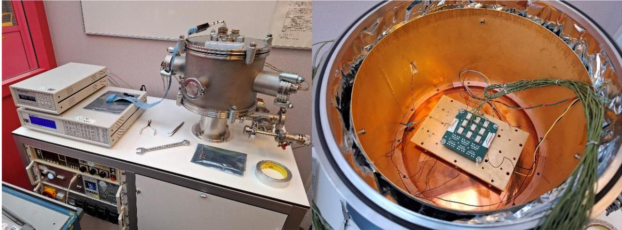
Fig. 4. BOXY cryostat external view (left) and BOXY internal view showing installed test PCB (right)
